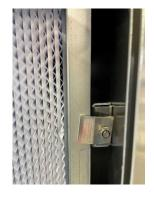
Remove all 4 filter tab retaining nuts remove the filter tabs and set aside. Slide the HEPA filter out along the filter guides and remove it from the machine. ALWAYS TREAT THE USED HEPA FILTER AS HAZMAT AND PROCESS IT ACCORDING TO YOUR ESTABLISHED HAZMAT PROCEDURES.
