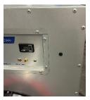
The OA2500 model's pressure sensor can be adjusted after removing the black plug. This calibration can be done while the machine is running. Using a piece of cardboard, cover about half of the back (intake) area of the machine – Figure 2 (below). As you slide the cardboard to cover more of the machine, the change filter light should go on when about 80% of the full intake is covered. You can use a small flat head screwdriver to adjust the sensor to ensure the light turns on at that point.
