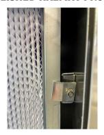
To replace the HEPA filter ensure that the gasket on the HEPA filter faces inwards toward the flange, slide the filter in place along the filter guides and re-install the filter tabs and filter tab securing nuts. Tighten the tabs so that the gasket is compressed approximately ½ of the thickness. This allows for the filter to be reseated and tightened at a later time if necessary.
