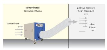
To create **NEGATIVE PRESSURE** inside the containment, more air must be exhausted compared to air entering the containment area. Place the machine inside the containment and hook a flexible duct to the outlet ring of the machine exhausting to outside the containment. (See Above) All of the air being exhausted has gone through the filters.
