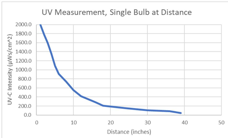
Figure 2: Reduction in UV radiation as the microorganism moves further away from the UV-C source. Bulb Type: Philips TUV TL Mini (16W 4P-SE).
